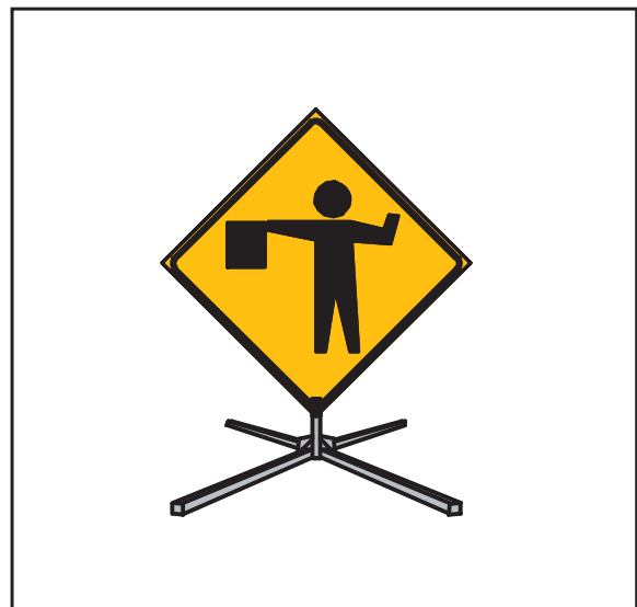
Figure H-2. Short-Term and Short-Duration Sign Mount (Daytime and Non-Regulatory Sign Use Only)
